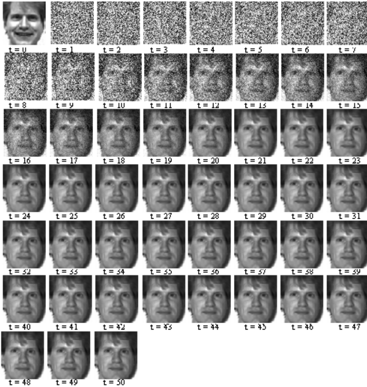
Fig. 4.42. A sample sequence of a progressive facial pattern recalling scheme performed by the Lee-associator
